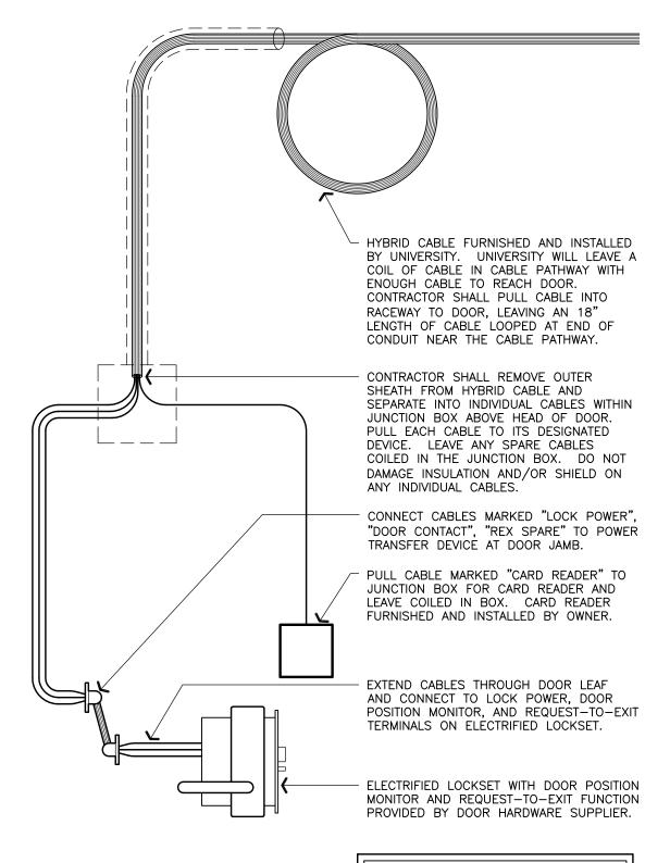
CONTRACTOR SHALL COORDINATE THE INSTALLATION AND TERMINATION OF WIRING WITH THE DOOR HARDWARE SUPPLIER AND UNIVERSITY NETWORKING AND TELECOMMUNICATIONS AND SHALL ASSIST IN COMMISSIONING THE ACCESS CONTROL SYSTEM.
